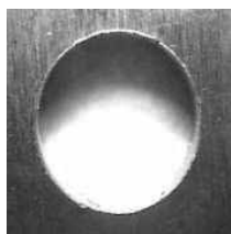
Class Two Feather burrs can be seen without magnification. They can be removed with your fingernail.
